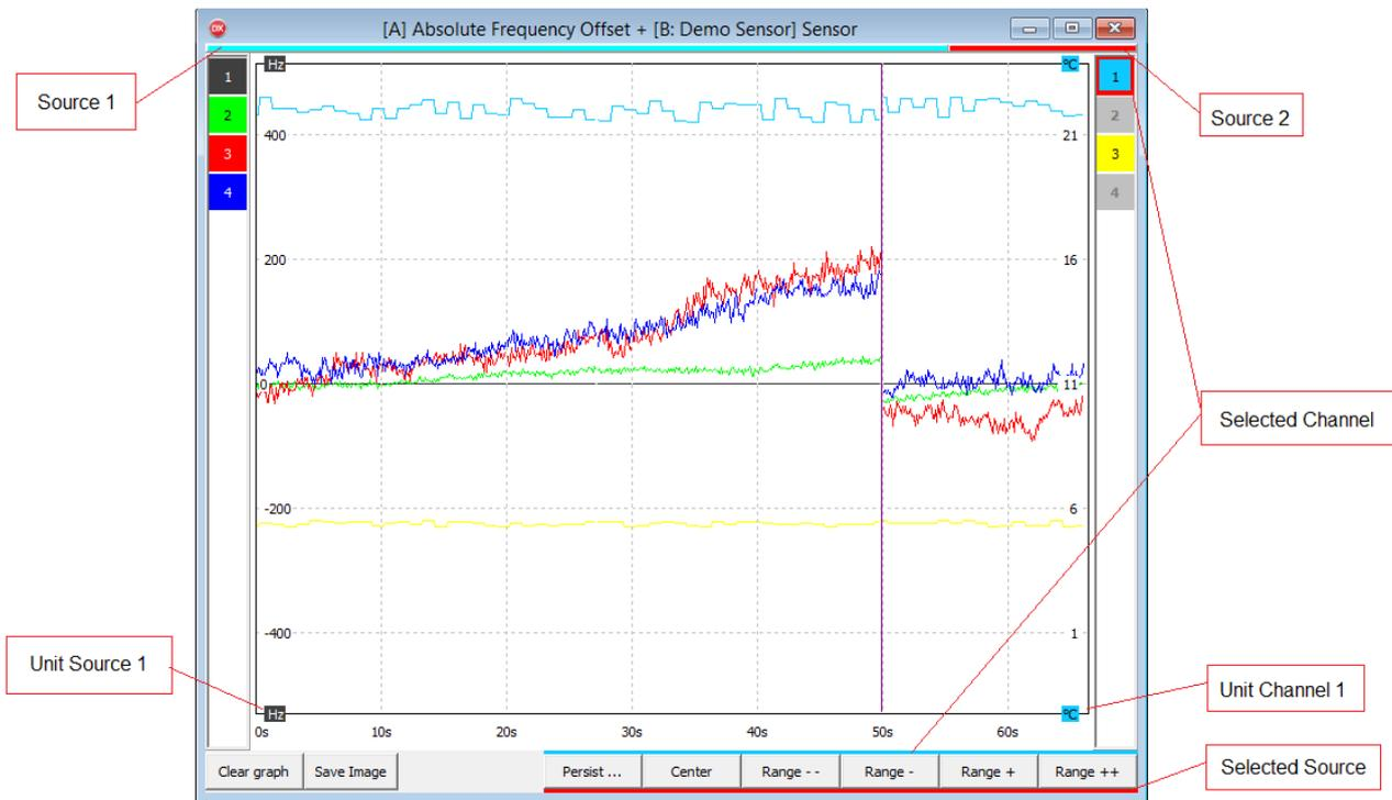
For the second source, the channel selection and scaling of this source is also shown on the right. Since there are devices that can provide different measures (such as temperature and humidity sensors), the scaling for each channel can also be set separately.
