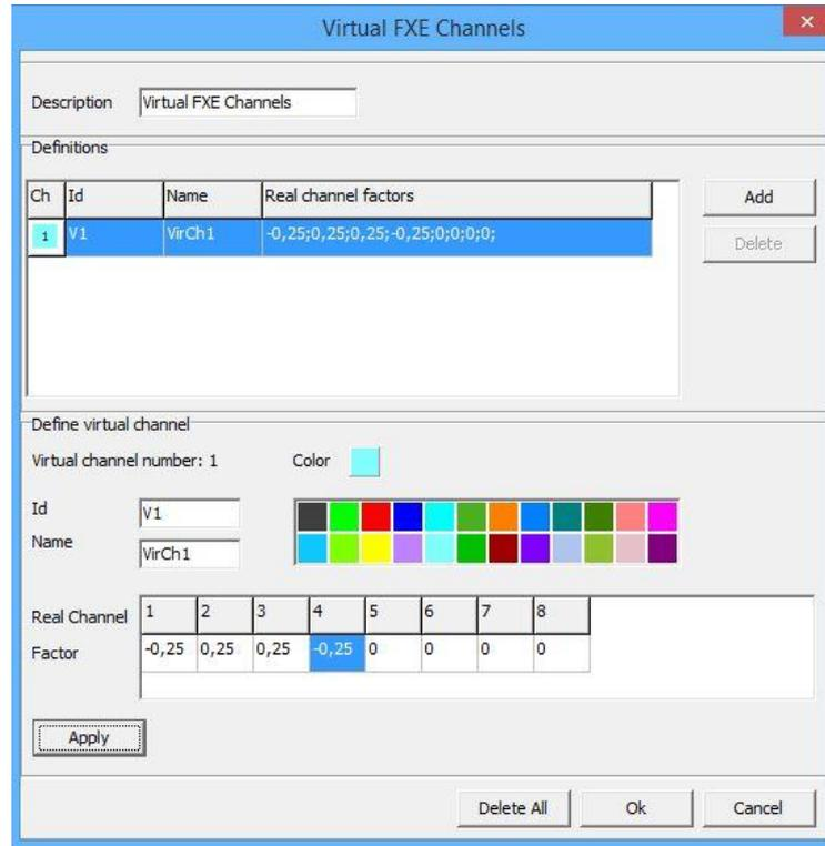
Definition of "virtual channels", i.e. linear combinations of the input data. The virtual channels can be displayed in text and graphic windows and output in log files. In the example a virtual channel  $VirCh1 = 0.25 * (-Ch1+Ch2+Ch3-Ch4)$  is defined.
