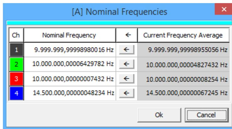
For each channel, an ideal frequency (nominal frequency) can be defined, which is used for the phase residual (deviation of the phase from the ideal value) or the relative frequency in relation to the ideal value. The value can be entered or an estimated value can be adopted.
